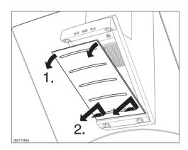
■ To remove the air intake panel gently pull out and downward, shifting the lower part a bit to the right. Lift it out of the latches.
